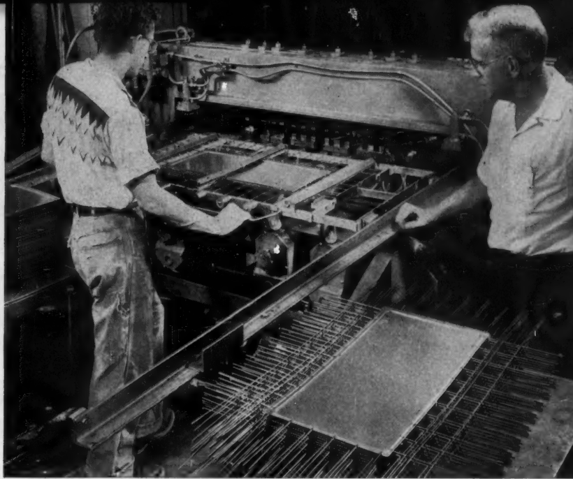
On this automatic multi-welder , design-specified by William Cannell, right, Bauer Bros. Co. master mechanic, a total of 288 different combinations of welds can be made. Here the operator is welding wire to a solid bottom basket for use by a major appliance manufacturer.
